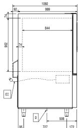
Drain ΕI = Electrical inlet (power)
